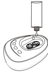
2. Place basket into tank, and fill the lens care solution (or physiological saline, purified water) into the upper edge of the stainless steel tank. Do not overfill.
