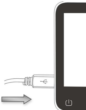
2、 Turn on the APEX LOCATOR, insert other end of data transfer cable into APEX LOCATOR
