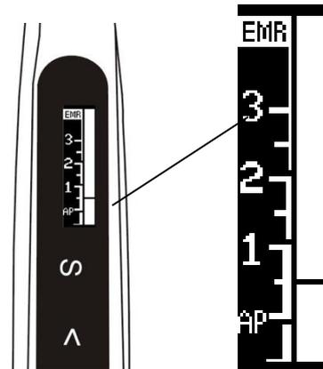
1. Insert the file into contra-angle handpiece, now contact the lip clip to file (short circuit).
