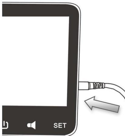
1. Insert the measuring wire into socket as shown in left picture, make sure connect properly
