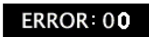
Error code 00 , means overload , motor is over current , should reduce the load.
