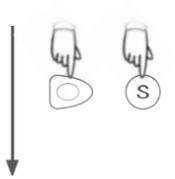
1. When the device is shutdown press key S and main switch at the same time.
