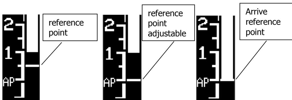
The position of the reference point is automatically setting with the APEX LOCATOR, and the cursor is displayed on the E-CONNECT screen.
