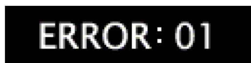
Error code 01 , means the continuous operation time is too long , motor is over heated, stop using the device for some time.
