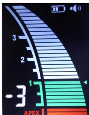
3. Observing APEX LOCATOR display, the root canal length strip will be all lighted, and a rapid beep sound will be generated at the same time, the 'APEX' sign will be flashed. That means the APEX LOCATOR is working normally.
