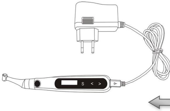
Connect the handle and adapter as shown.
