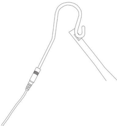
2. Check the measuring wire, file clip, lip hook and APEX LOCATOR are connecting properly. Make file clip hook with lip hook (short circuit)
