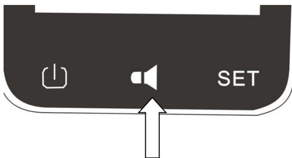
The APEX LOCATOR's volume of the key and alarm sounds can be adjusted. Press the volume keys to cycle the volume through the minor to the maximum.
