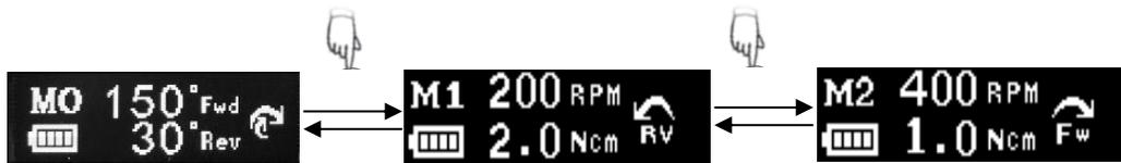
E-CONNECT has 10 memories(M0 to M9) , users can set the memory(combine different speed, torque and reverse direction ) by themselves. Memory M0 is reciprocating mode, there are 5 units reciprocating degrees in M0, press S key to switch. M1-M9 are for normal mode.
